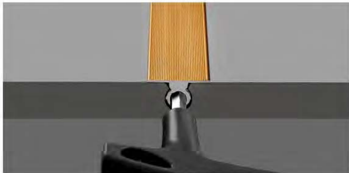
3. Decide the direction of rotation according to the bending of the door panel, and adjust with a hex wrench
